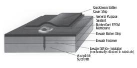
The batten strips, in turn, are anchored by Elevate fasteners and sealed with Elevate Fastener Sealer.
