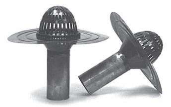
Long life drains consist of an 18" diameter, 20 oz. (0.27) spun copper flange, with slight corrugations, soldered to a seamless copper pipe. The flange is coated with a bituminous paint to ensure a good bond with the roof membrane. May be specified unpainted for use with generic materials other than asphalt.
