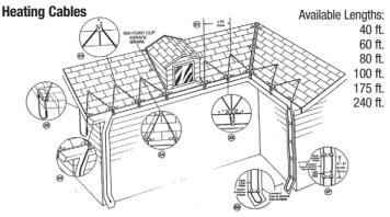
Great for eavestrough, roof edge, downspout de-icing and for melting a path for water flow to roof drains.
