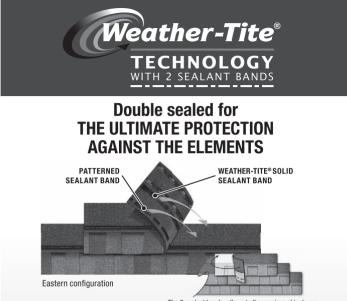
The 2 sealant bands adhere to the previous shingle row, providing double protection against the elements
