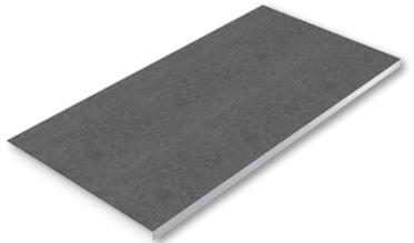
Closed-cell polyisocyanurate (polyiso) foam core integrally bonded to non-asphaltic, fiber-reinforced organic felt facers. Offered in a variety of thicknesses, providing long-term thermal resistance (LTTR) values from 5.7 to 26.8. Manufactured in accordance with ASTM C1289, Type II, Class 1, Grade 2 (20 psi) or Grade 3 (25 psi) and CAN/ULC-S704 Type 2, Class 3 or Type 3, Class 3.
