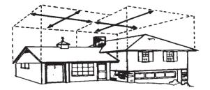
The minimum requirement to ventilate your home is 1 sq. ft. of ventilation for every 300 sq ft of ceiling area, except in cathedral or less than 2/12 pitch when 1 sq. ft. of ventilation is required for every 150 sq ft.
