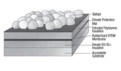
As a result, the roofing membrane is protected year-round from surface damage and severe weather conditions. This system is ideal for roofs with regular traffic or in severe climates.
