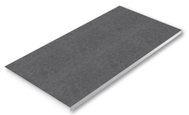
Closed-cell polyisocyanurate (polyiso) foam core integrally bonded to non-asphaltic, fiber-reinforced organic felt facers. Offered in a variety of thicknesses, providing long-term thermal resistance (LTTR) values from 5.7 to 26.8. Manufactured in accordance with ASTM C1289, Type II, Class 1, Grade 2 (20 psi) or Grade 3 (25 psi) and CAN/ULC-S704 Type 2, Class 3 or Type 3, Class 3.
