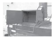
Automatic Temperature Controls – Your choice of fully automatic or semi automatic ini-lo provides maximum control and safety by maintaining asphalt at a consistent temperature.
