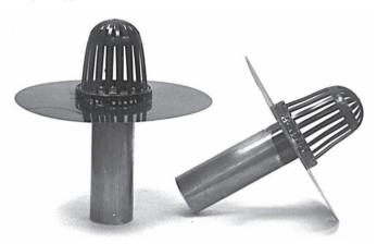
Long life drains consist of an 14" diameter, 16 oz. (0.22) spun copper flange, with slight corrugations, soldered to a seamless copper pipe. The flange is coated with a bituminous paint to ensure a good bond with the roof membrane. May be specified unpainted for use with generic materials other than asphalt.
